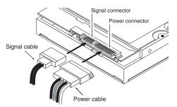
Each cable is keyed to ensure correct orientation. Pipeline HD drives support latching SATA connectors.
